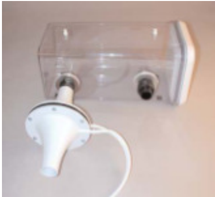
Figure 6: The rear panel of the GA-300 gas analyzer showing the inlet and outlet ports for the gas sampling tubing.
