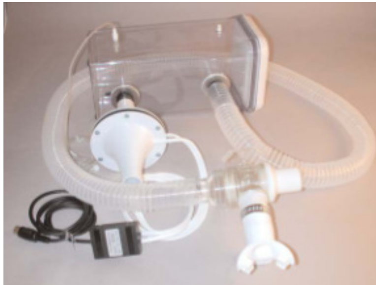
Figure 5: The spirometer circuit used to measure the volume of air exhaled by the subject, and provide oxygen and carbon dioxide samples from the exhaled air to the gas analyzer.
