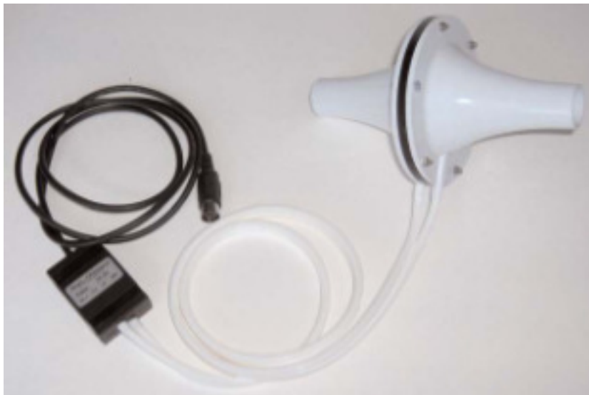
Figure 3: The A-FH-1000 flow head from the GAK-100 kit connected to the SP-304 spirometer with a pair of airflow tubes..
