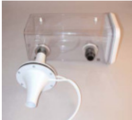
Figure 4: The inlet of the A-FH-1000 Flow Head attached to the outlet of the mixing chamber.
