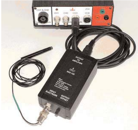
Figure 5: Dissolved oxygen electrode (ISE-730) and amplifier (DO2-100) connected to an IWX/214 with a male DIN-DIN cable.
