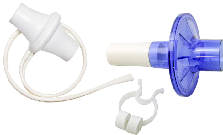
Figure HS-1-S1: The student respiratory kit and A-FH-300L flow head and the airflow tubing. The blue filter attaches to the flow head.
