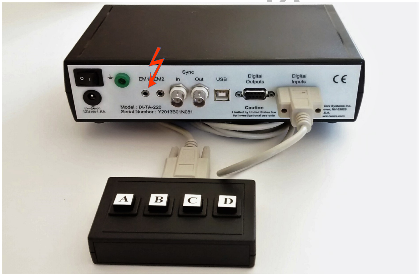
Figure HP-17-S3: The IXTA shown with the RPD-400. If using the EM-220 Event Markers, these will plug into the EM1 and 2 ports on the TA as shown.
