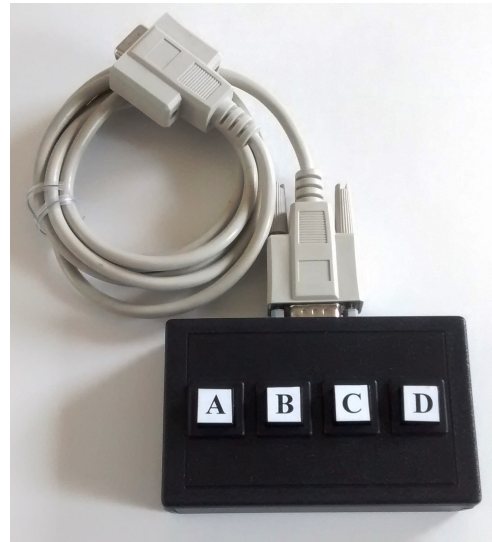
Figure HP-17-S2 RPD-400 4-Button Response Pad.
