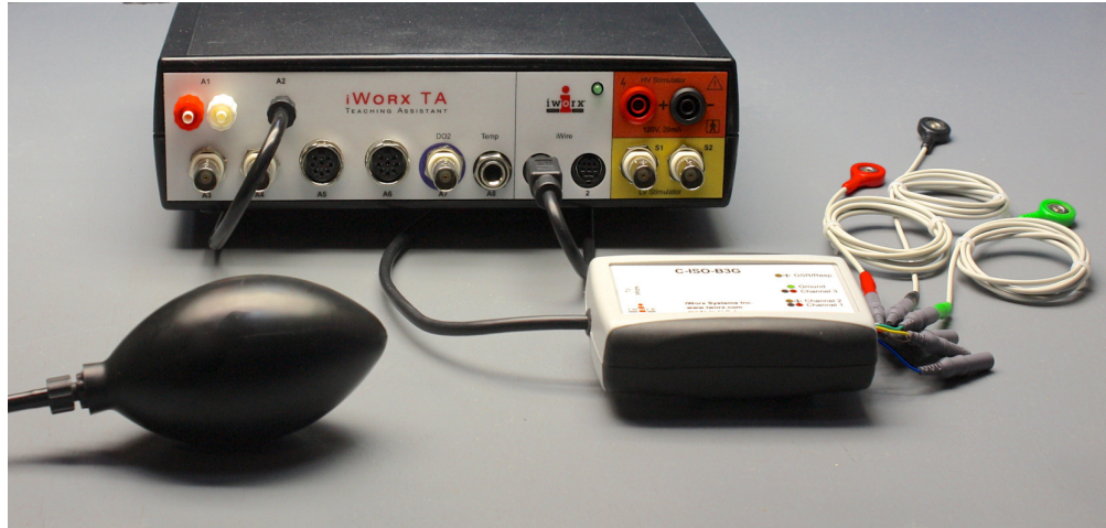
Figure HM-1-S3: The EMG cable and hand dynamometer connected to an IXTA
