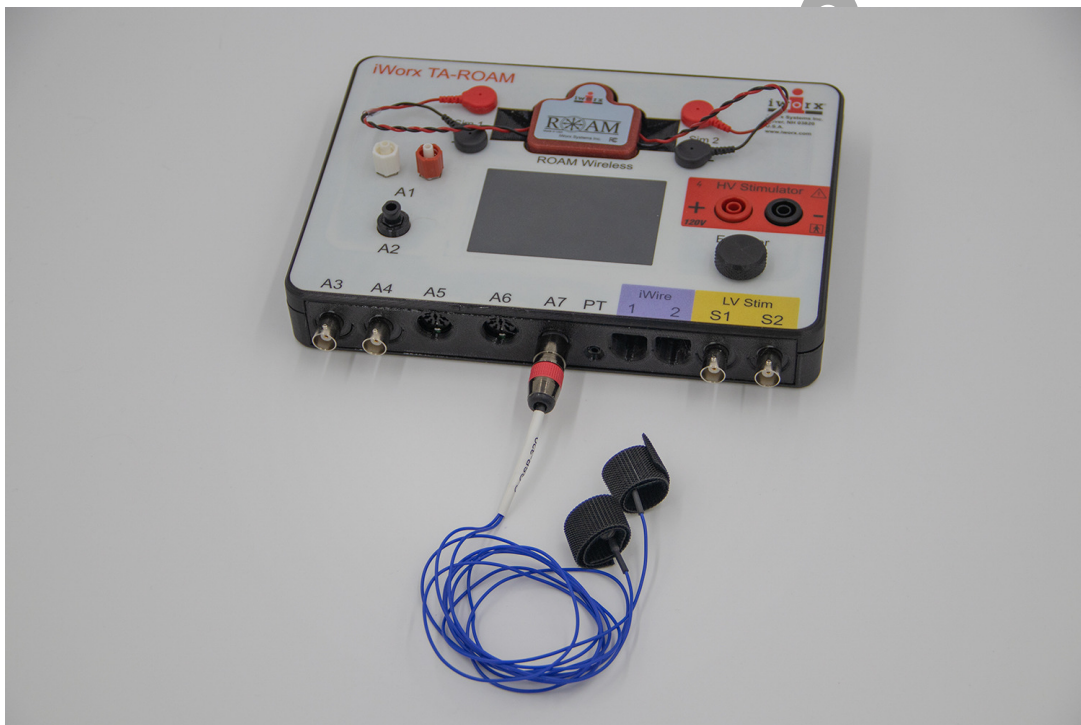
Figure HP-3-S1: The GSR galvanic skin response amplifier.
