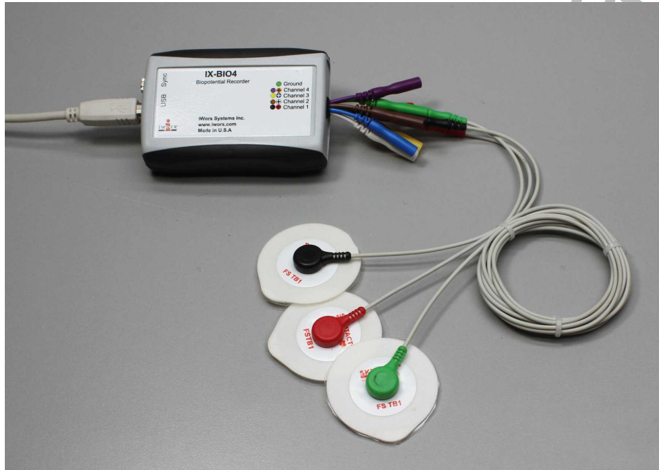
Figure HH-1-S1: The IX-BIO4 ECG cable with three lead wires attached.
