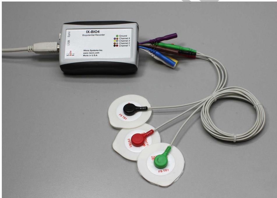
*Figure HH-2-S1: The IX-BIO4 with three lead wires and electrodes connected.*
