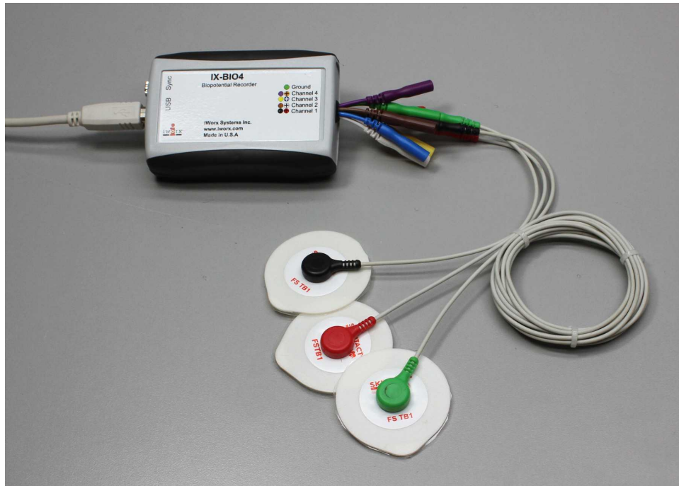
Figure HM-2-S1: The IX-BIO4 with three EOG lead wires and electrodes connected.
