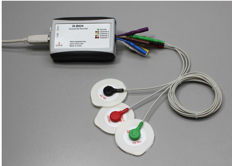
Figure HP-2-S1: The IX-BIO4 with three snap leads for use with disposable electrodes attached.
