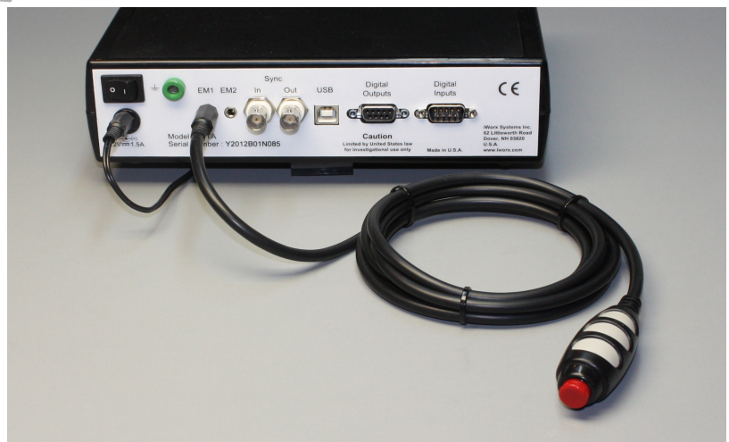
Figure HP-23-S2: The IXTA with the EM-220 event marker.
