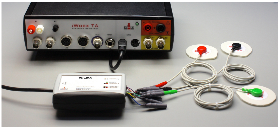
Figure HP-23-S4: iWire-B3G EOG cable attached to the front of the IX-TA.
