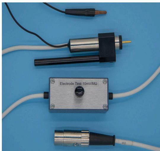
Figure AN-1-S1: The IC-200 intracellular probe.
