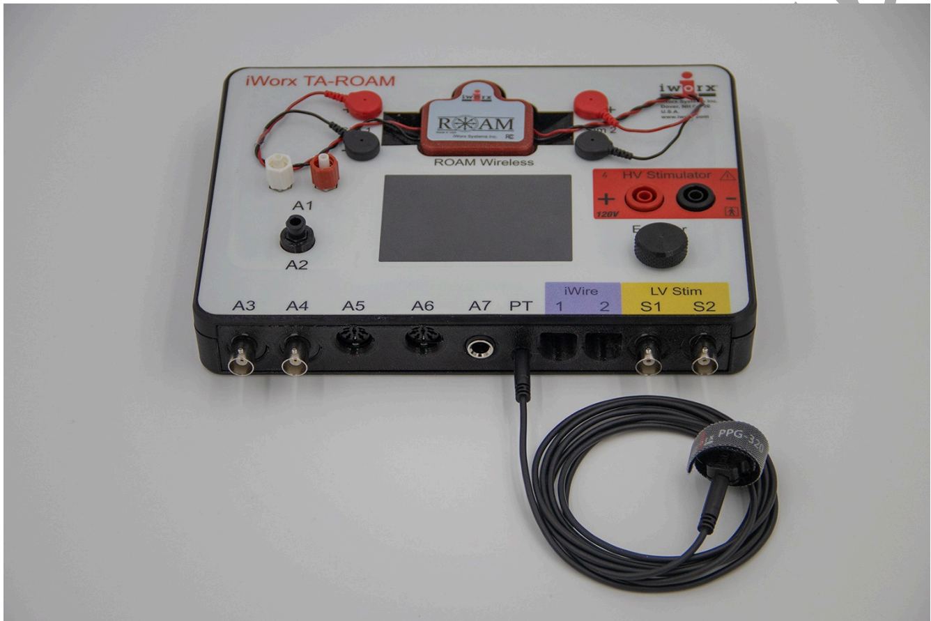
Figure HE-1-S1: The PPG pulse / temperature sensor connected to the TA data recorder.
