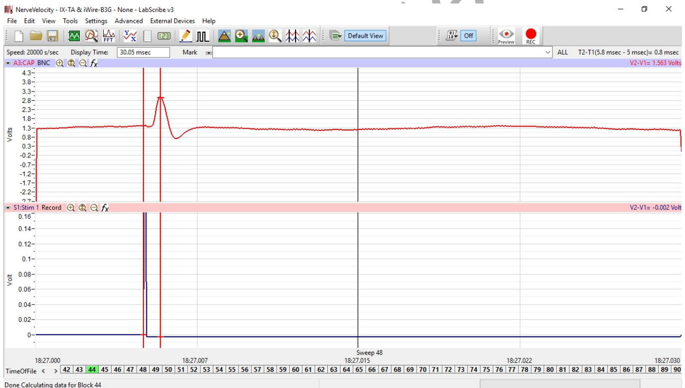
Figure HN-122-L1: A CAP from the median nerve; measuring the amount of time between the initial stimulus and the peak voltage.
