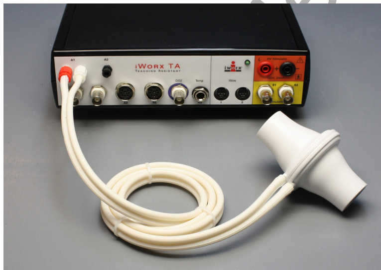
Figure HS-9-S3: The flow head connected to the internal spirometer of the IXTA unit. The USB Pulse oximeter will be connected directly to the computer.
