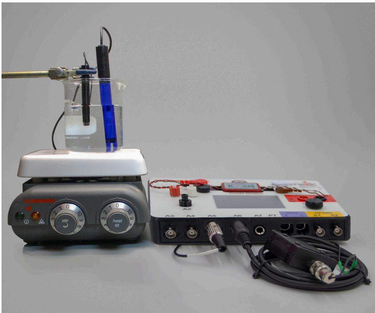
Figure GB-3-S3: The setup for recording oxygen concentration levels and pH using the iWorx/IXTA.
