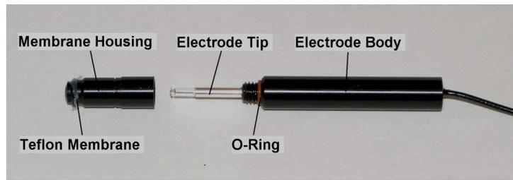
Figure GB-3-S1: The dissolved oxygen electrode, shown with its membrane housing removed. The end of the housing is covered with a Teflon<sup>(tm)</sup> membrane secured in place by an O-ring. The platinum wire inside the glass tube is the cathode and the silver sleeve that surrounds the glass tube is the anode.
