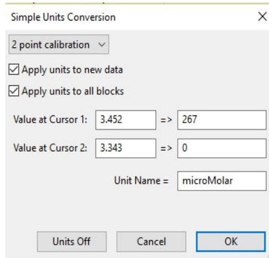
Figure GB-3-S6: The Simple Units Conversion dialogue window with the voltages at the cursors set to equal the dissolved oxygen concentrations used in calibration.
