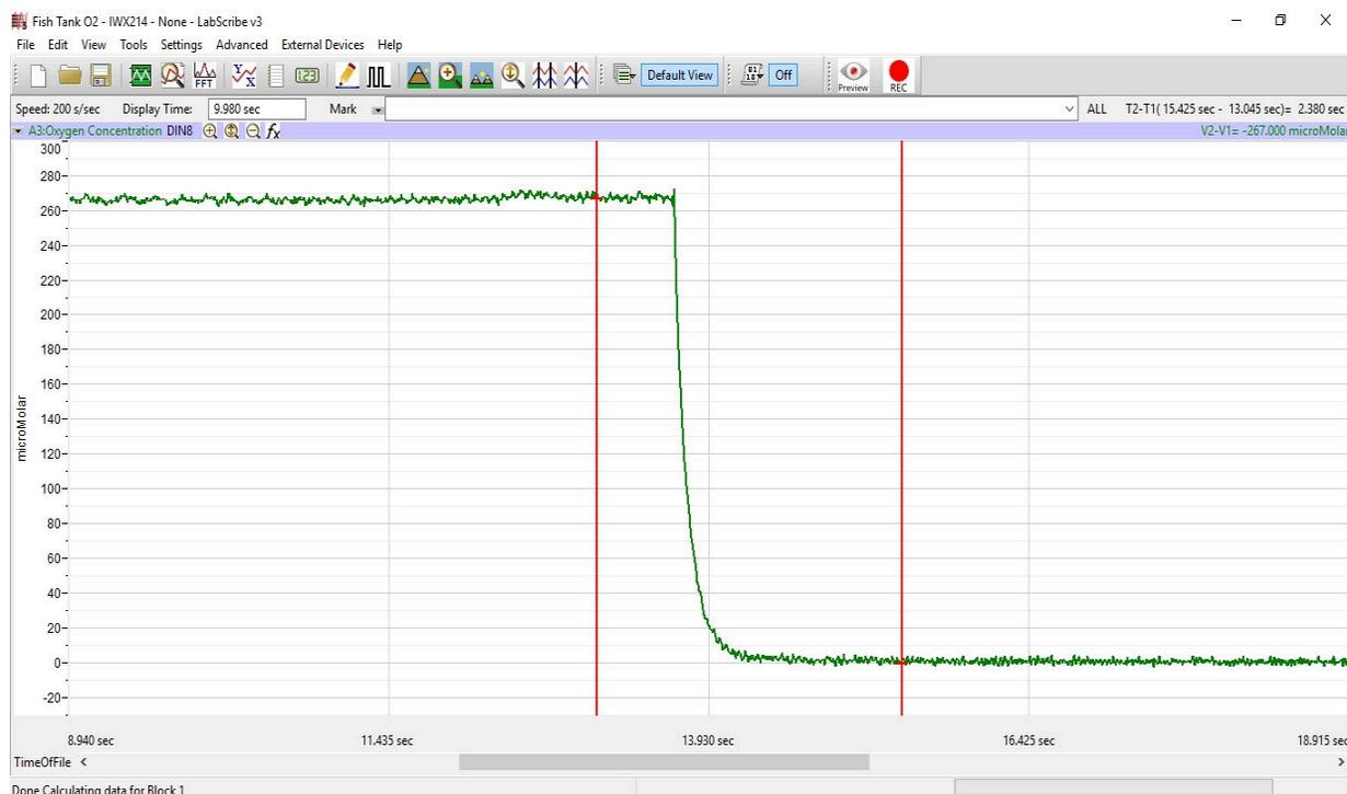
Figure GB-3-S5: Recording of oxygen concentrations in air saturated and oxygen depleted deionized waters used to convert the units of the Y-axis from voltage to  $O_2$  concentration ( $\mu$ Molar).
