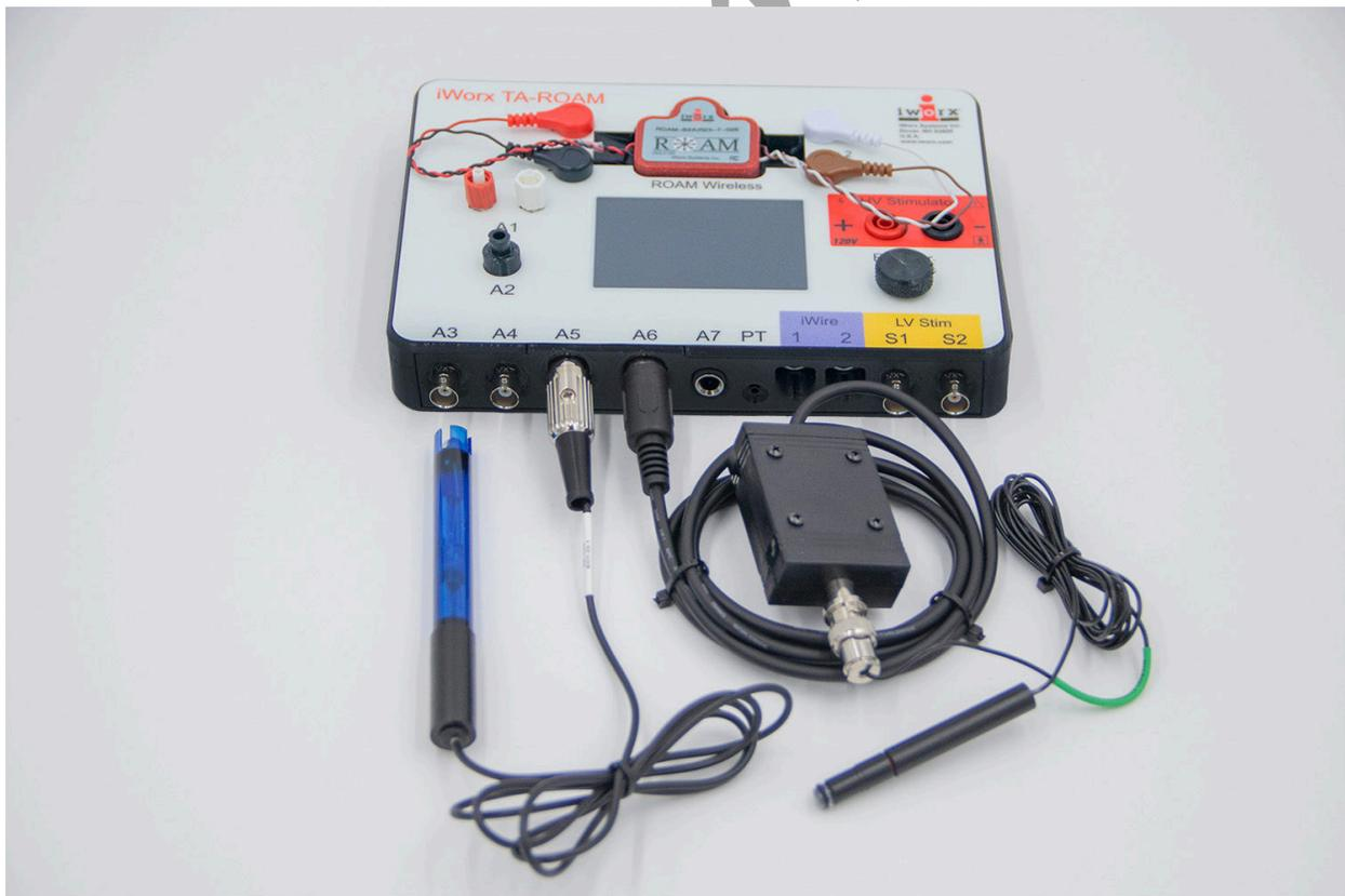
Figure GB-3-S2: The dissolved oxygen probe and pH probe connected to the IXTA.
