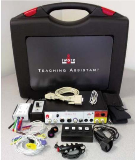
The kit includes a data recorder and all of the sensors needed to record physiological signals and perform cognitive and normative analyses.
