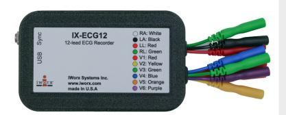
Measuring all 12 ECG leads simultaneously, this compact and lightweight ECG recorder enables highly detailed analysis of the anterior, lateral and inferior regions of the heart. The IX-ECG12 connects to and is powered by a USB port on any Windows or Macintosh computer. Data is recorded and analyzed with iWorx advanced LabScribe ECG Software Module
