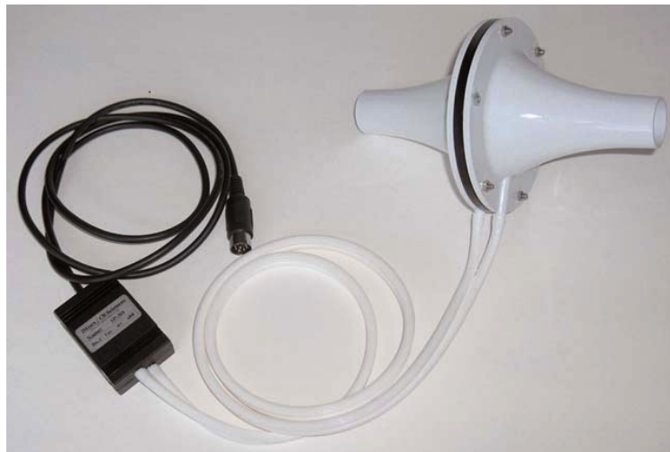
A-FH-1000 Flowhead, connected to the SP-304 Spirometer
